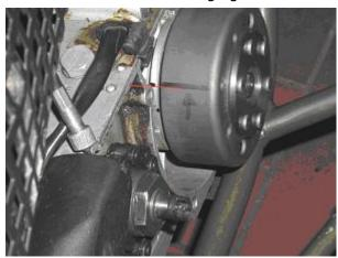
Take the spark plug out and bring the piston into ignition position. Might be 2mm BTDC.
