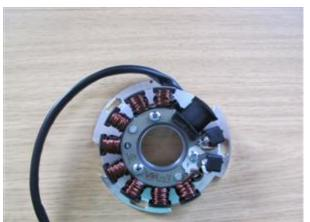
Have a look at the new stator unit. You will find there a little left from the larger black coil a small red marking. This is an ignition marking for timing.
